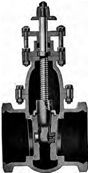
FIG. 109.—Eddy Gate-valve (taper-seat, double-gate).
